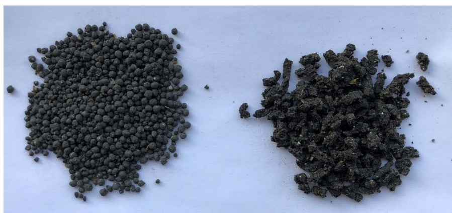
Pictured: Pellets from a rotary drum dryer (left) and dried biosolids from a belt dryer (right)
