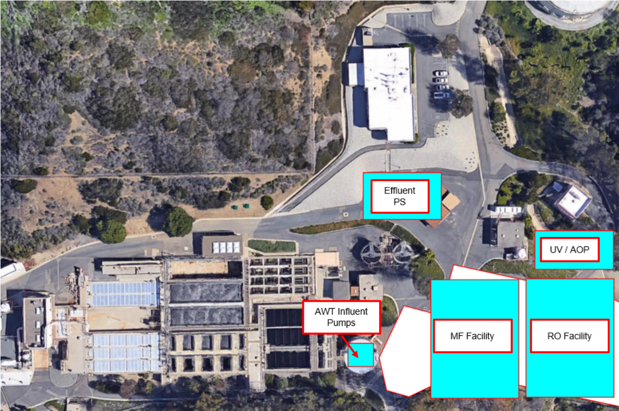
Figure 7-4. Example Site Layout of Advanced Water Treatment Facility for BNR or AGS Alternatives
