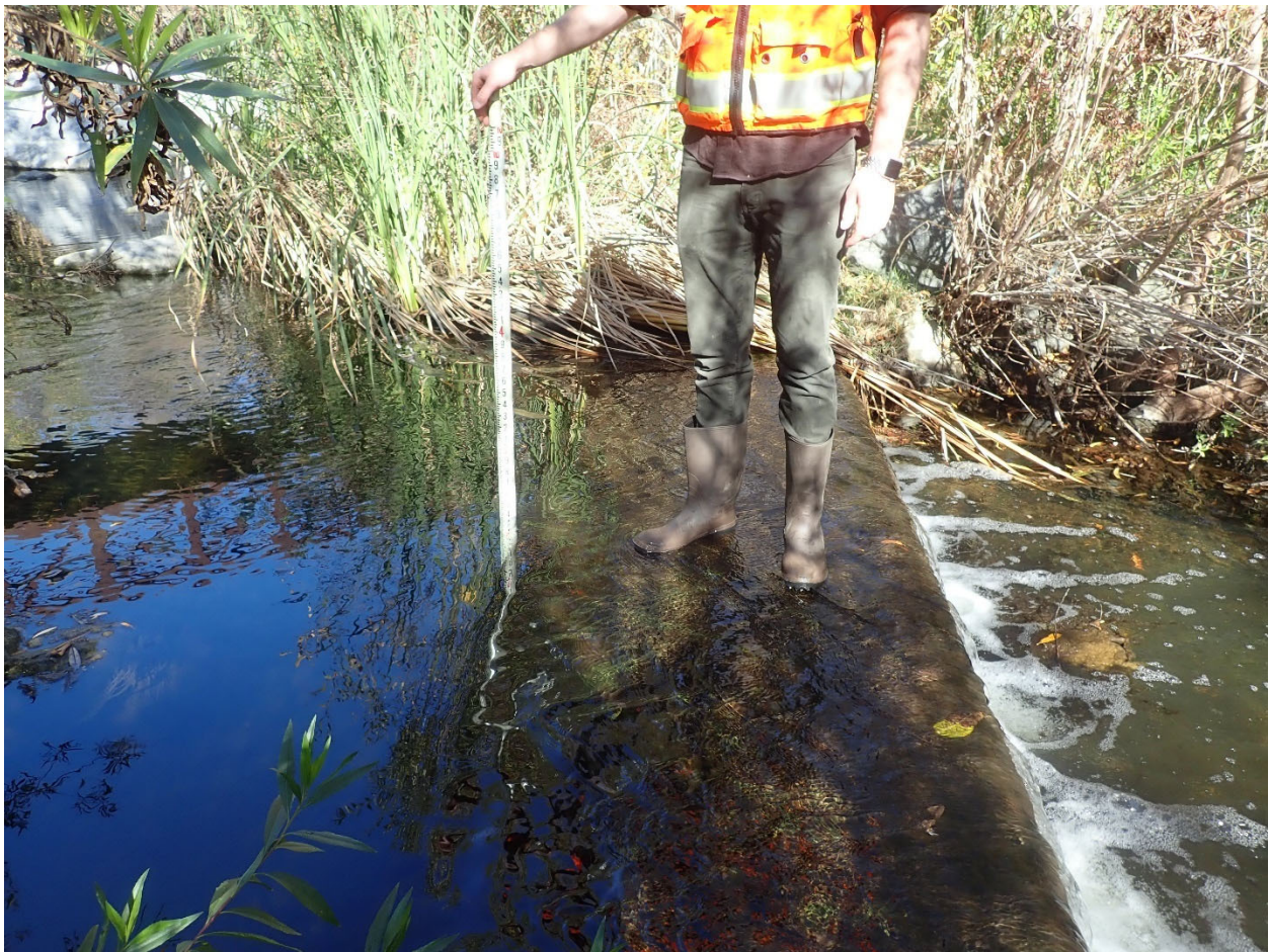
Figure 2.1 – Measuring the Creek Bottom along the ETM Encasement in 2023
