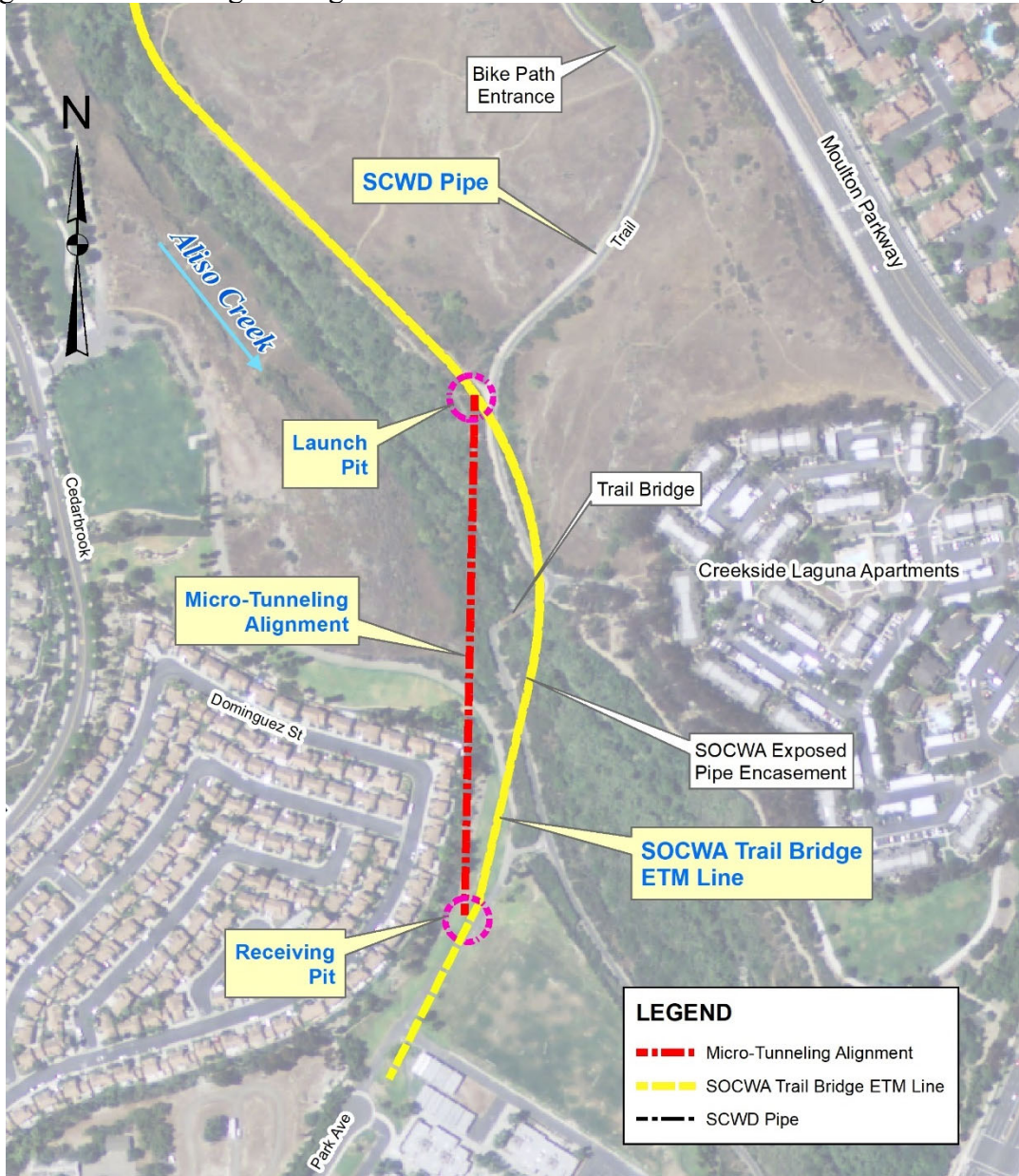
Figure 3.1 – Approximate Alignment of Micro-tunneling Segment
