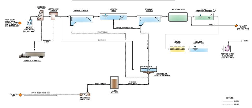
Flow Schematic 3 - Los Alisos Water Reclamation Plant
